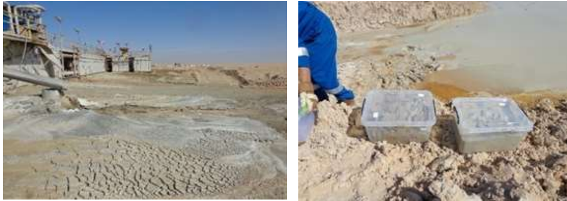
Figure 2.3. Water based mud sample collection and preservation
