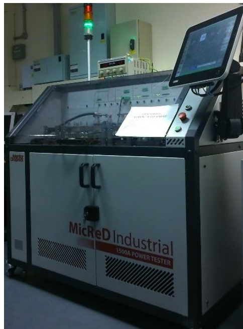
Figure 4.1 Mentor Graphics 1500A Power Tester used for the power cycling test and transient impedance measurement.
