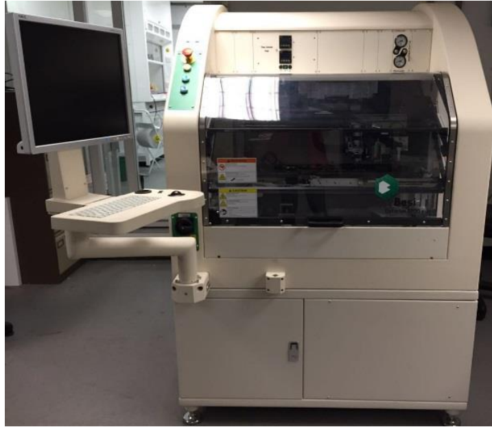
Figure 3.9 Photograph of a Datacon 2200 EVO die bonder used for pressure-assisted sintering process and die placement.
