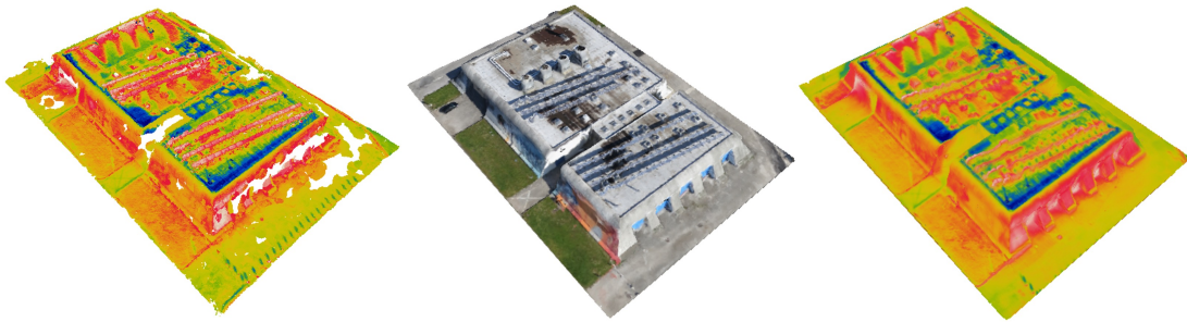
Figure 2.10: A 3D TIRpoint cloud, 3D RGB mesh model and resulting 3D textured thermal model using ICP for 3D-3D fusion (Maset et al., 2017).
