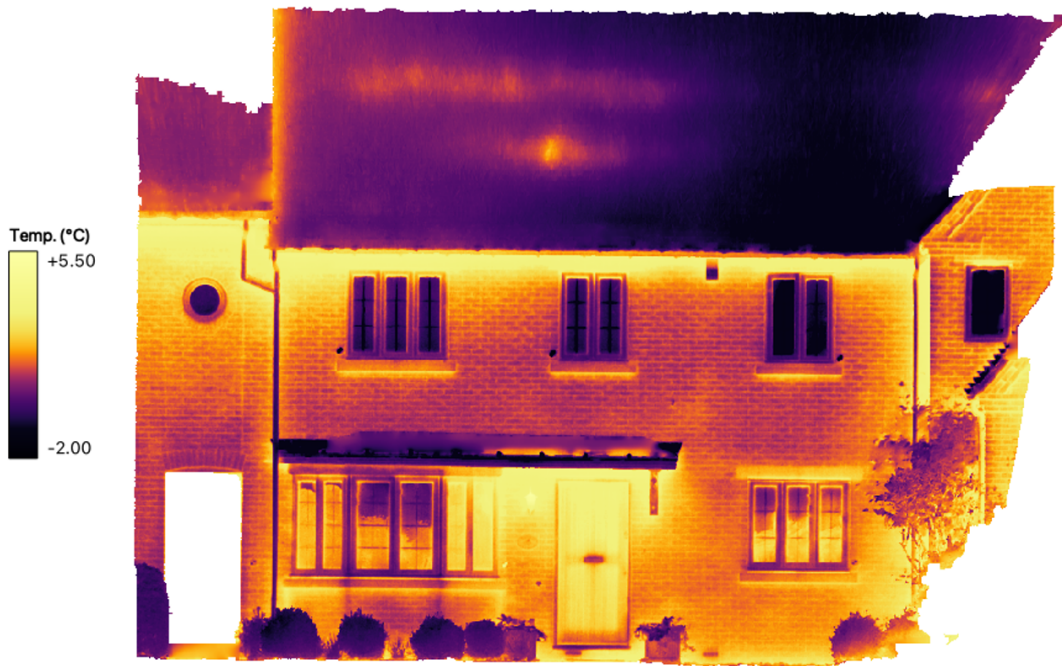
Figure 5.15: Quantile thermal orthomosaic for Dunrobin House
