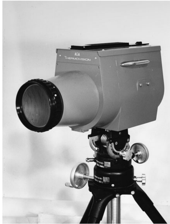
Figure 3.2: Agema Infrared Systems’ AGA Thermovision 665 (1965-1967), one of the first commercial, mass production, single-element sensor, optomechanical scanner thermal cameras (Rogalski, 2012; Vollmer & Möllmann, 2018).
