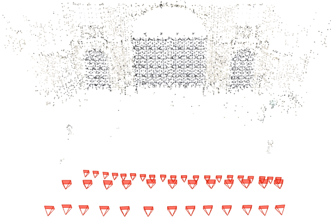
Figure 4.11: Combined TIR-RGB bundle block adjustment camera network for Lenton Lodge Gatehouse, showing the single strip of WWP images and two strips of RGB1 images.
