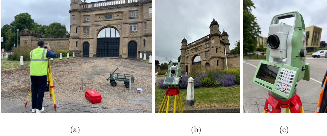
Figure 3.19: (a, b) Geodetic survey of Lenton Lodge Gatehouse, including (c) the Leica TS10 total station.
