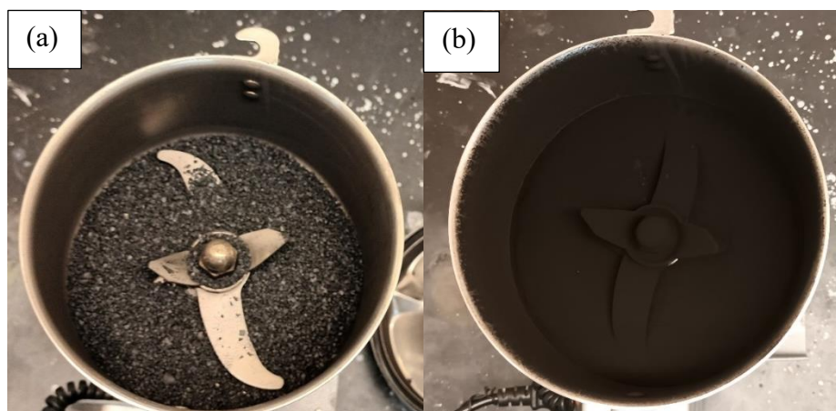
Figure 3.5 Visual comparison between the (a) original particle size and the (b) powdered form of palm kernel shell after grinding.
