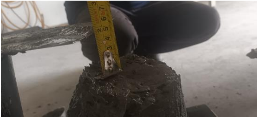
Figure D.2: Concrete mix with 4% 500°C PKS.
