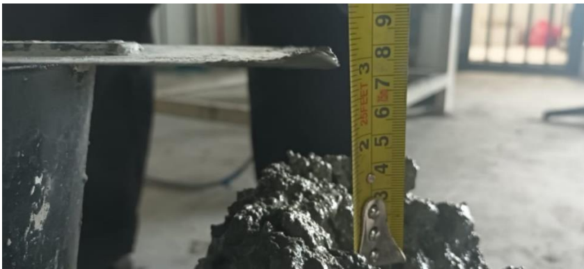
Figure D.3: Concrete mix with 4% 409°C PKS.
