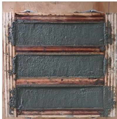
Figure 4.4 Biochar mortar composites casted for 40 × 40 × 160 mm.
