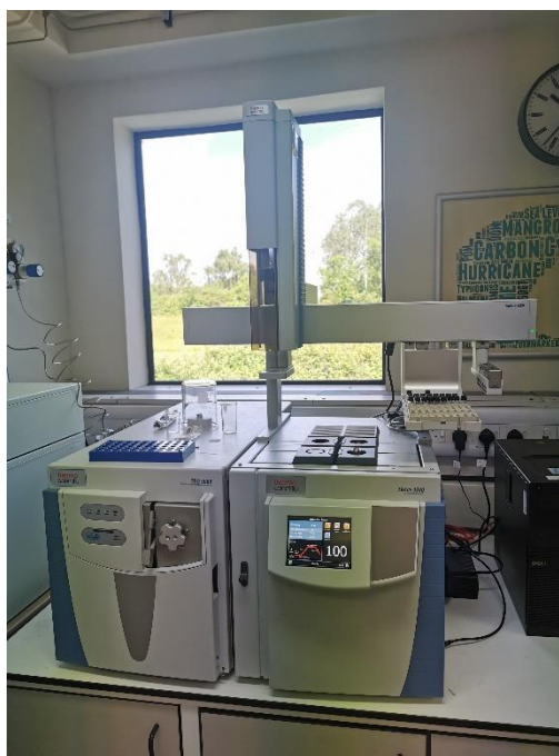
Figure 14: Thermo Scientific Trace 1300 gas chromatograph (GC) coupled to a Thermo Scientific TSQ9000 mass spectrometer (MS).
