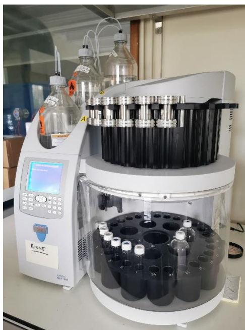
Figure 12: Dionex™ ASE 350 used for PAH extraction from soils.
