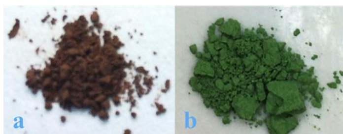
Figure 5.2.13 TPP@NbP via different immobilisation time. Mixing 30 mg TPP and 1 g NbP catalyst in 15 mL TOL for a) 24 hours shows brown colour; b) 0.5 hour shows green colour.
