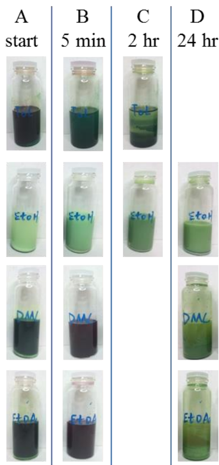
Figure 5.2.5 The immobilisation process of TPP on NbP catalyst in different solvents (30 mg TPP and 1g NbP catalyst mixed in 15 mL of each solvent separately: Tol, EtOH, DMC and EtOAc. Column A: just adding NbP catalysts; Column B: stirred for 5 min; Column C: stirred for 2 hour; Column D: stirred for 24 hour. The immobilisation processed in Tol finished quickest among these four solvents. And the immobilisation did not accomplish in EtOH after 24 hour.
