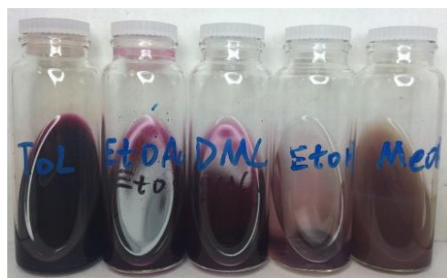
Figure 5.2.4. 30 mg TPP in 5 mL of different solvents (methanol (MeOH), ethanol (EtOH), ethyl acetate (EtOAc), toluene (Tol) and dimethyl carbonate (DMC)). TPP has highest solubility in Tol, and the brown MeOH solution is not ideal solution for further investigation.
