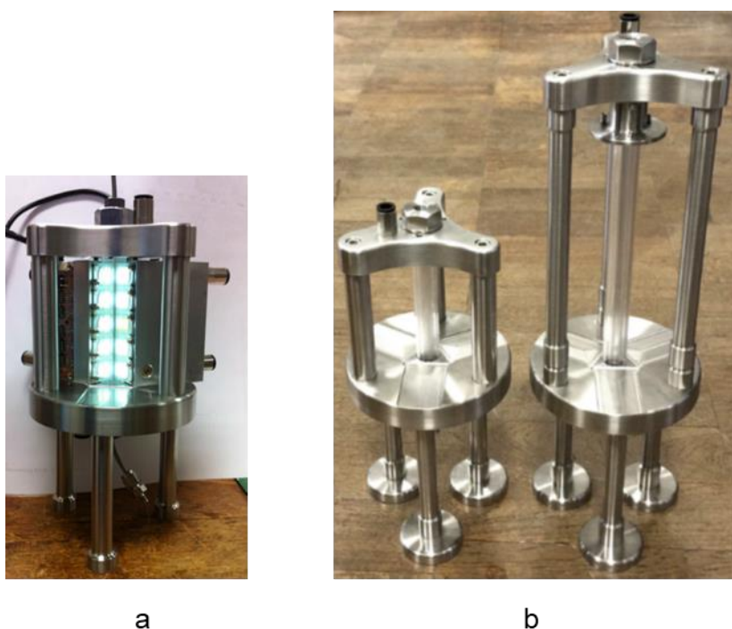
Figure 2.3.2 Photographs of sapphire tube photoreactors. Picture a shows the sapphire tube reactor is held in the centre of photoreactor and is exposed by LED blocks (actually 3 LED blocks can be fitted, but for the easy exhibition, there were only 2 LED installed when the photo was taken). Picture b show a small and a larger volume reactors.
