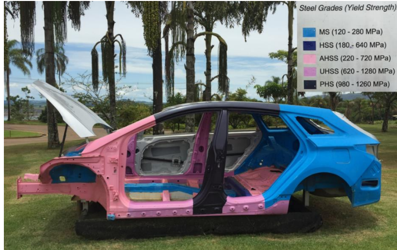
Picture 1.1.1.2 The car - body steel structures using different niobium micro-alloyed steels. The coloured parts represent the niobium containing steels made in different strengths. (Author's photo taken in CBMM, Araxá, Brazil)
