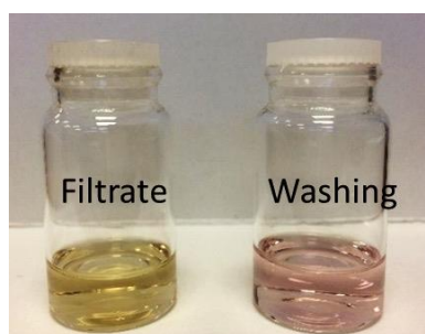
Figure 5.2.3 The collection of filtrate and of washing EtOAc solution after the immobilisation process, The coloured solution indicated that not all the TPP was immobilised on the NbP catalyst and that there was TPP leaching from the NbP support.
