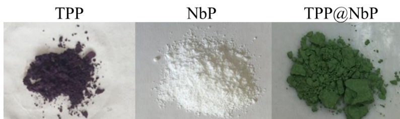
Figure 5.2.2 Photosensitiser TPP (purple), NbP solid acid (white) and bifunctional catalyst TPP@ NbP (green).
