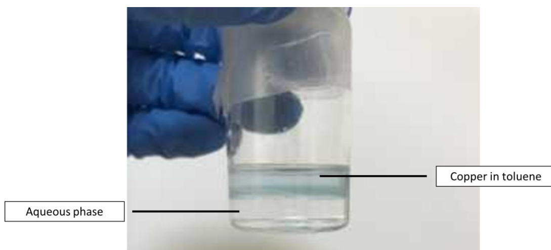
Figure 6.2 Photograph of successful transfer of copper ions from aqueous phase to toluene.
