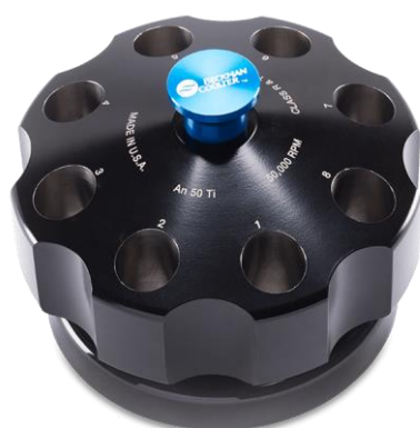
Figure 3.2 An 8 hole rotor (a) and cell (b) of an AUC
