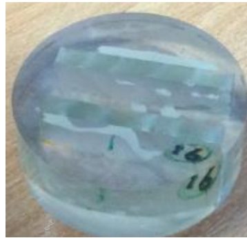
Figure 6.12 Specimen prepared for optical microscopy
