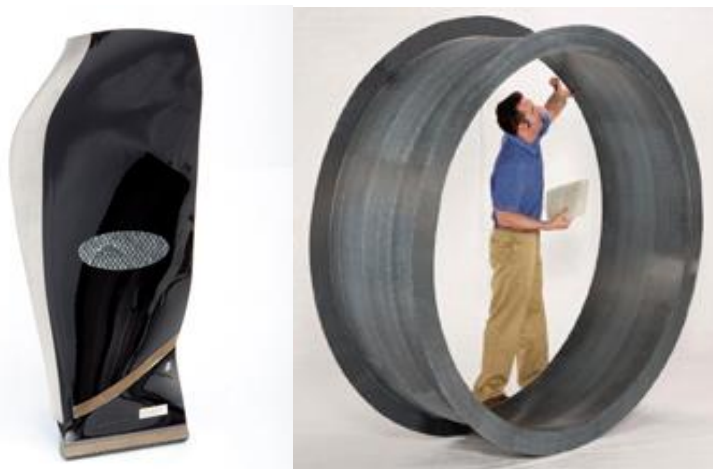
Figure 2.8 Composite fan blade (left) [35] and composite fan containment case (right) [34] developed with 3-D woven technologies. Note that fibre damage can occur during the weaving process. Usually this damage is caused by the repeated actions of abrasion and bending when yarns go through the loom, or yarn-to-yarn friction and loss of sizing agent, especially when using fibres which are fragile and with high friction coefficient such as glass fibres. Some researchers [36, 37] found that the accumulation of damage during weaving can lead to the loss of mechanical properties such as tensile strength of composites. Thus, various solutions are proposed to minimize fibre degradation, including use of additional sizing agent on fibres to lower yarn friction. Fibre sizing also possesses other essential functions such as protecting the fibres from environmental erosion, strengthening the bond between fibres and resin matrix, and improving the wettability of fibres during flow [38]. Fibre size should be specific to each type of resin system, as it must dissolve from the resin during forming process.
