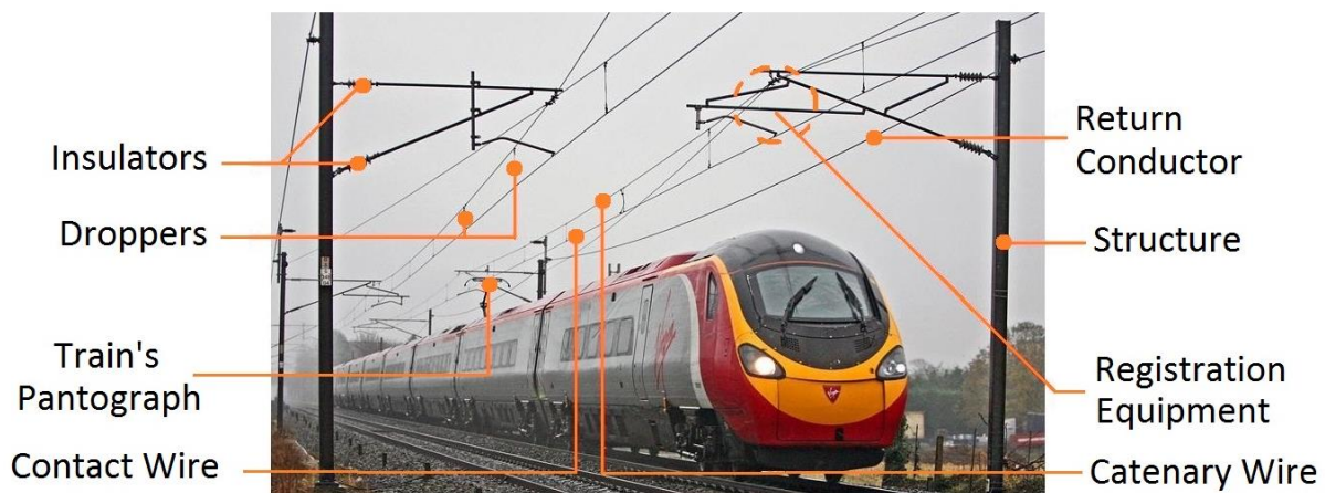
Figure 2-4 The Main OLE Components
