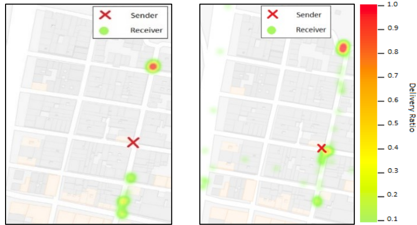
Figure 5.7b Single hop communication in dense city centre area of Valencia for 2.4 Ghz and 5 Ghz respectively.
