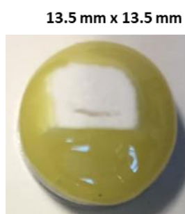
Figure 5.8. Representative hydrated tablet with a small crack near the base of the cross-section.
