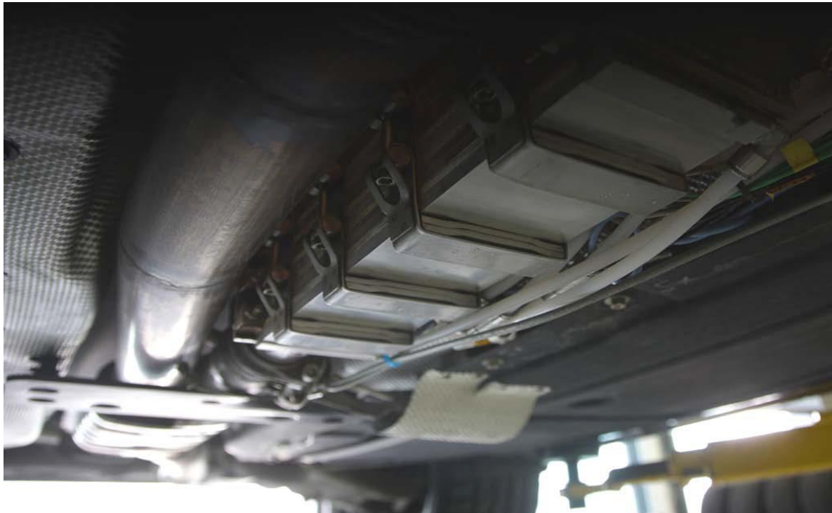
Figure 2-2 Bi 2 Te 3 TEG(2007) and High Temperature TEG, P max =300W (2009).
