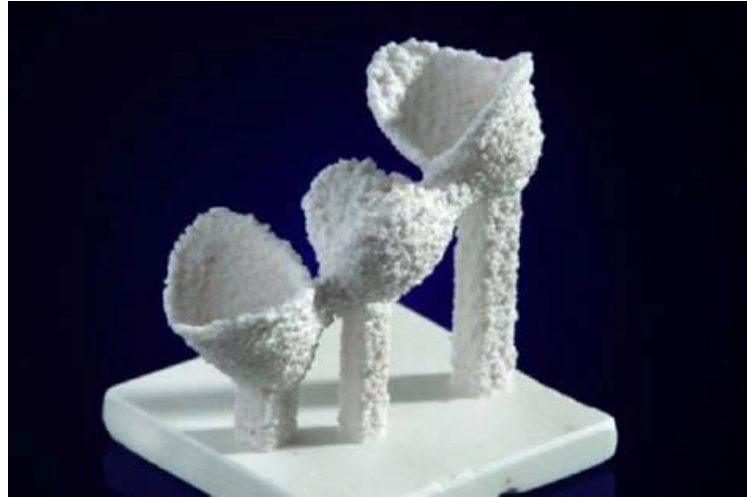
Figure 2-11: As-built Zirconia-Alumina component made by SLM (Wilkes et al., 2013).
