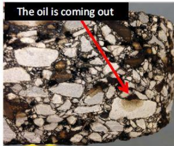
Figure 2.34: Asphalt sample after cyclic loading with broken capsules (Garcia et al., 2015).
