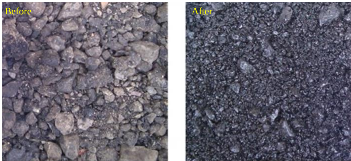
Figure 2.12: Asphalt mixture before and after the application of rejuvenators (Macismo, 2012).
