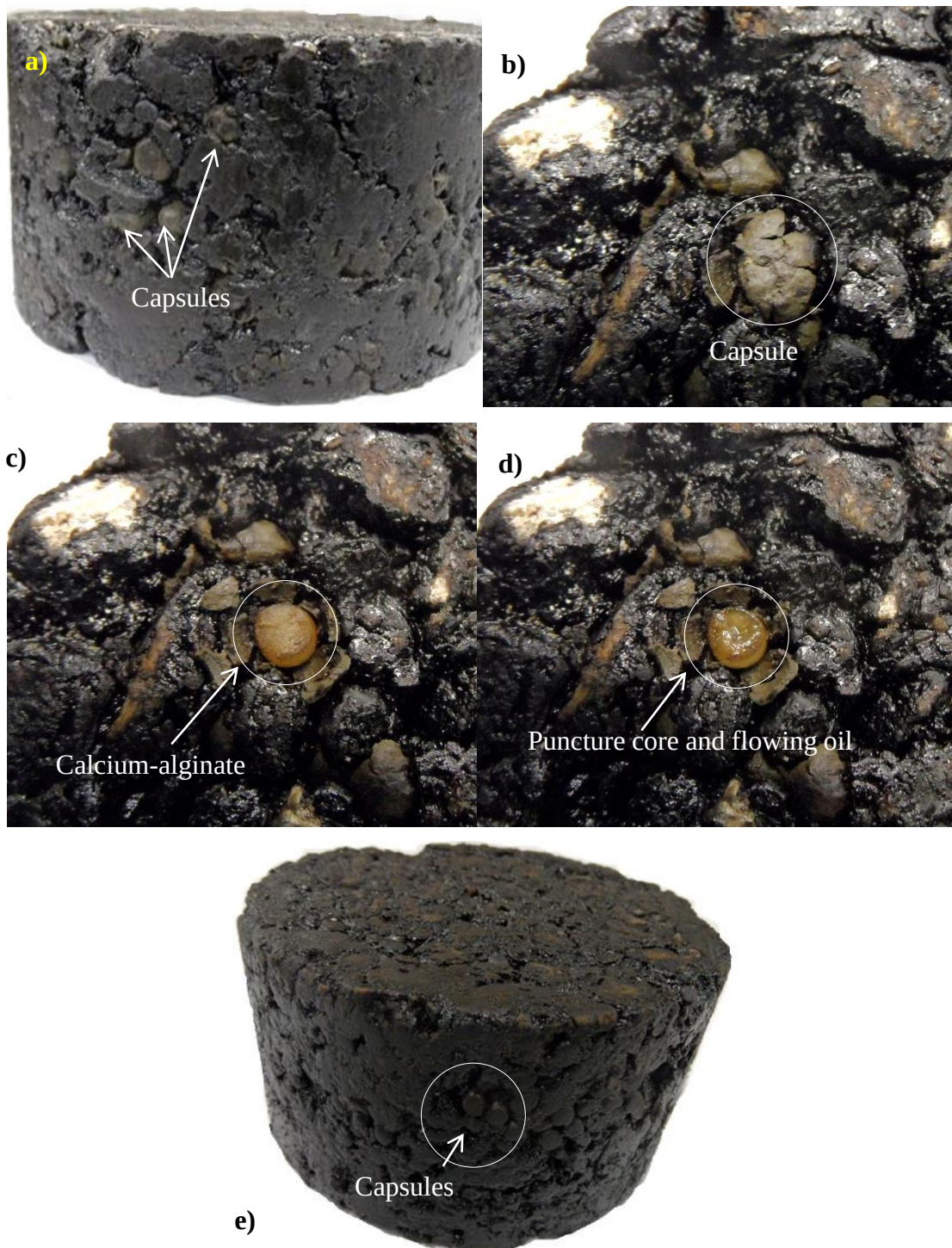
Figure 3.8: Images of asphalt specimens with capsules, (a) overall image of a test specimen with capsules with hard shell; (b) zoom-in of a capsule on top surface; (c) capsule with epoxy-cement shell removed; (d) the oil flowing from the capsule; (e) overall specimen with capsules without a hard shell.
