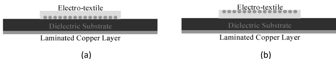
Figure 3.1: Cross sectional schematic of a satin weave fabric microstrip resonator for when (a) the conductive threads are placed underneath and (b) on top of the nonconductive threads [62].
