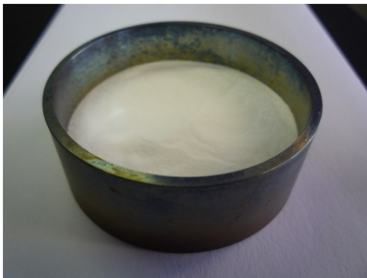
Figure 1. The BMW elastomer powder placed in the stainless steel cup before measurement.
