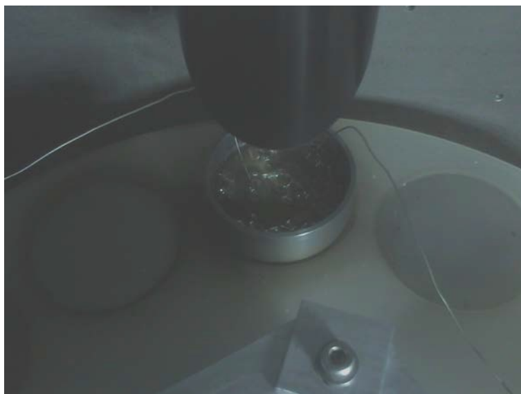
Figure 10. The Elastomer powder boiling at 200° C
