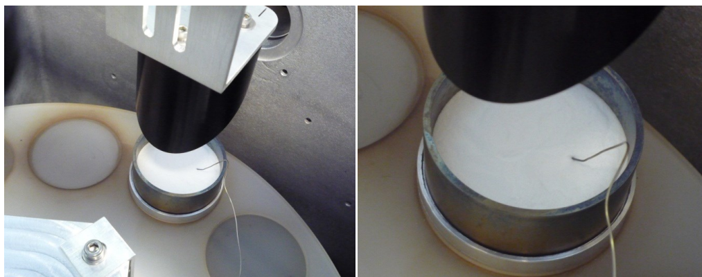
Figure 2. The cup with BMW elastomer and temperature sensor in the emissivity chamber.
