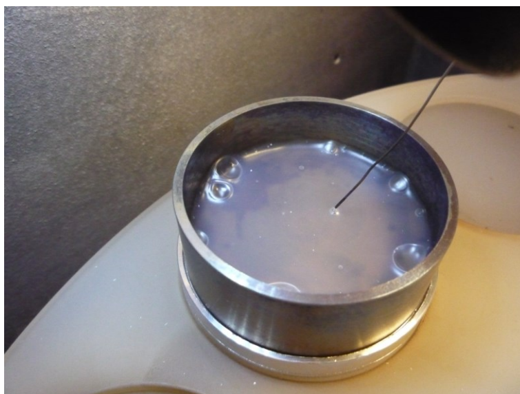
Figure 3. BMW elastomer in the steel cup after melting and cooling.
