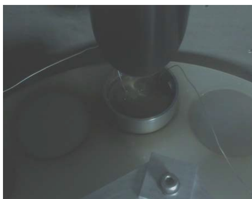
Figure 11. The Elastomer powder back at 125° C after melt (a, left), and its calibrated emissivity spectra (b, right)
