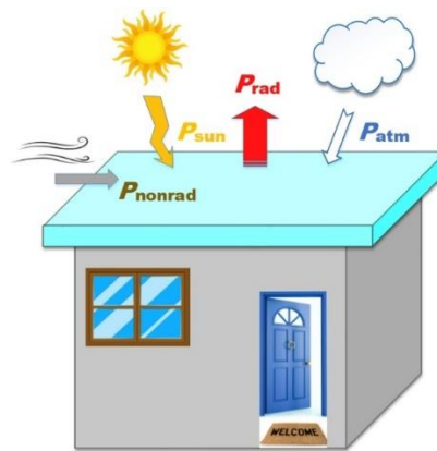
Figure 2-10 Schematic diagram of roof RC in a building (Chen and Lu, 2020).
