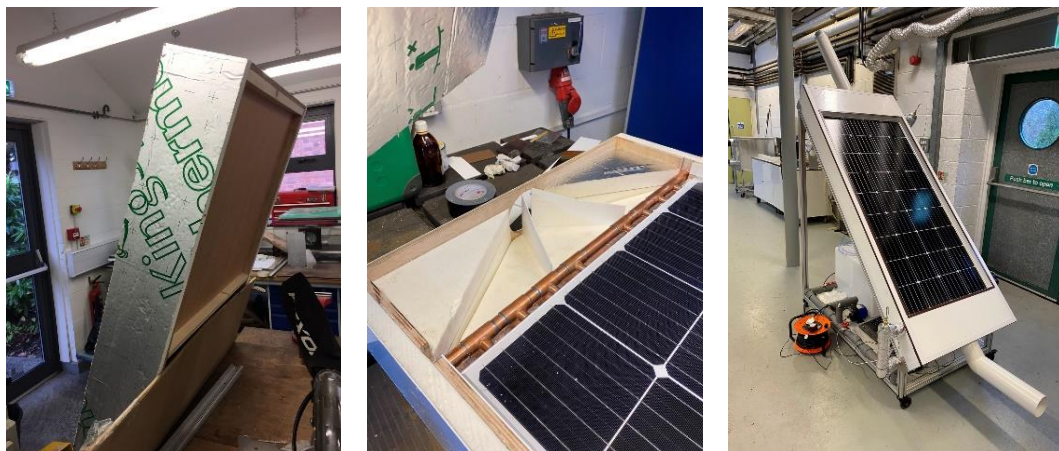
Figure 7-8 Construction and preparation of the PVT-RC module to be connected to the experimental system. See the flow separator structure marked in the image above.
