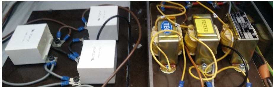
Figure 6.2: Photograph of input filter of the matrix converter
