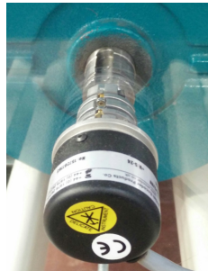
Figure 6.10: Photograph of encoder mounted on the motor shaft
