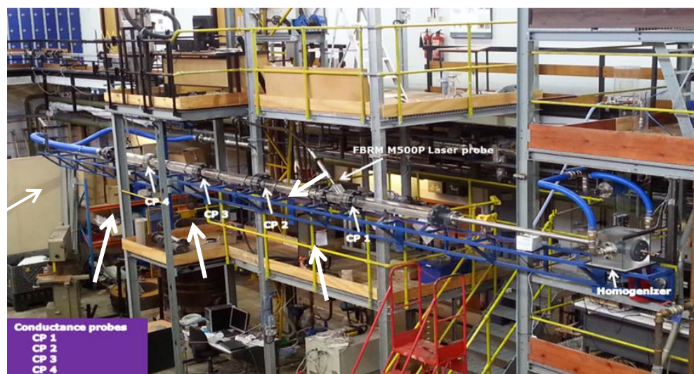
Liquid – Liquid Horizontal Flow Pipeline Sudden Expansion Rig in L3 Main Laboratory, Process and Manufacturing Engineering, Faculty of Engineering, Nottingham.
