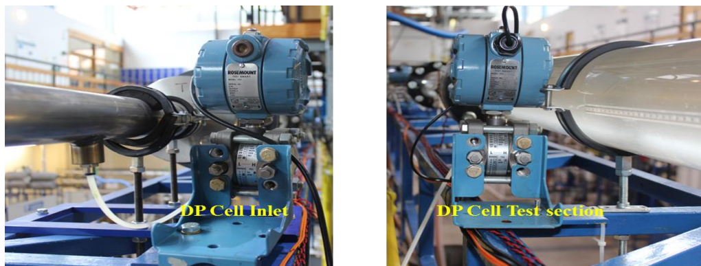
Figure 4-17 Photograph of Differential pressure transducers installed on the rig.
