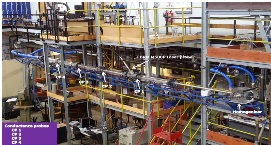
Figure 4-8 Liquid – liquid horizontal flow pipeline sudden expansion rig in L3 Main Laboratory,
