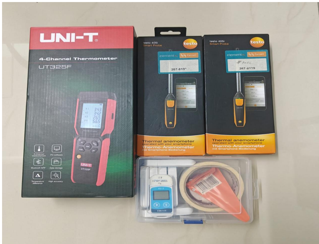
Figure 3.10. Temperature and wind condition measuring device used during the experiment
