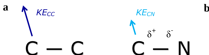
Figure 2.3: An illustration of the initial state effects observed for two different carbon environments, in which the bonding environment of the photoelectron emitter affects the photoelectron kinetic energy, which in turn affects the apparent binding energies of the C 1s photoelectrons. The fact that the carbon in (b) is in an electropositive environment makes extraction of electrons more difficult, resulting in lower photoelectron kinetic energies than in neutral (a) or electronegative carbon environments.
