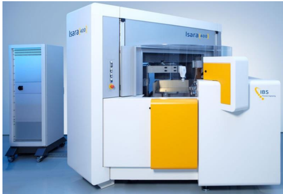
Figure 2-5: Photograph of Isara-400 ultra-precision CMM manufactured by IBS Precision Engineering [23].
