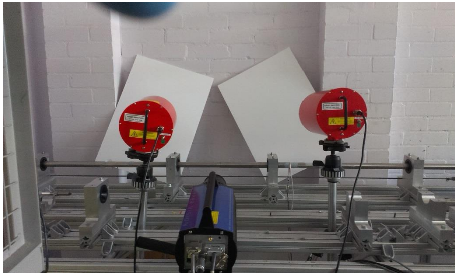
Fig 4-13 Arrangement used for capturing images during SHPB testing
