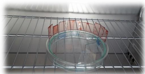
Figure 4-7 Oven treatment of the sol gel coated glass substrates
