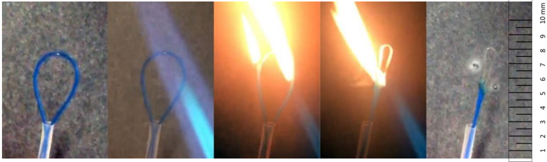
Figure 3-3 U-shape optical fibre sensor fabrication process via burning, photographs from left to right. Fiber shaping and fixation, burner on, burning procedure start, shaping the fibre under the heat exposure, red U-shape with scaling ruler
