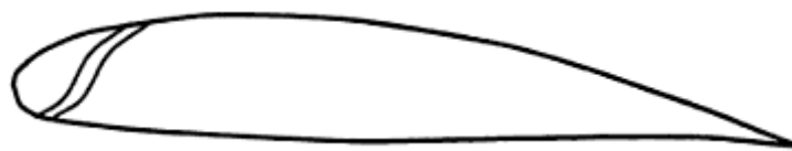
Figure 2-8 Leading-edge slot (Roskam and Lan, 2003)
