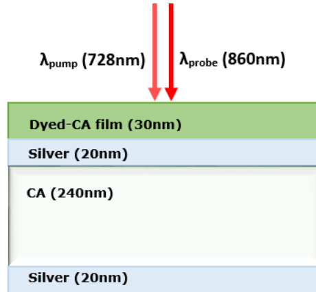
Figure 110: Schematic of a hybrid device with a dielectric absorbing dye-CA layer with 30nm thickness and CA-based spacer. The pump at 728nm and the probe at 860nm are used for excitation and detection, respectively.
