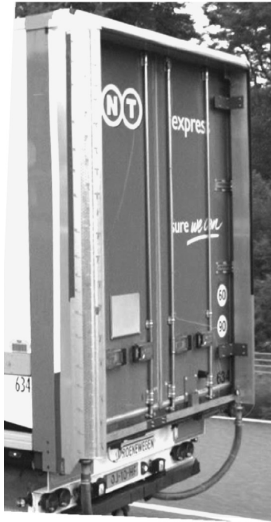
Figure 2.10: Curved overhangs on the rear of the truck to promote the conada effect [49].
