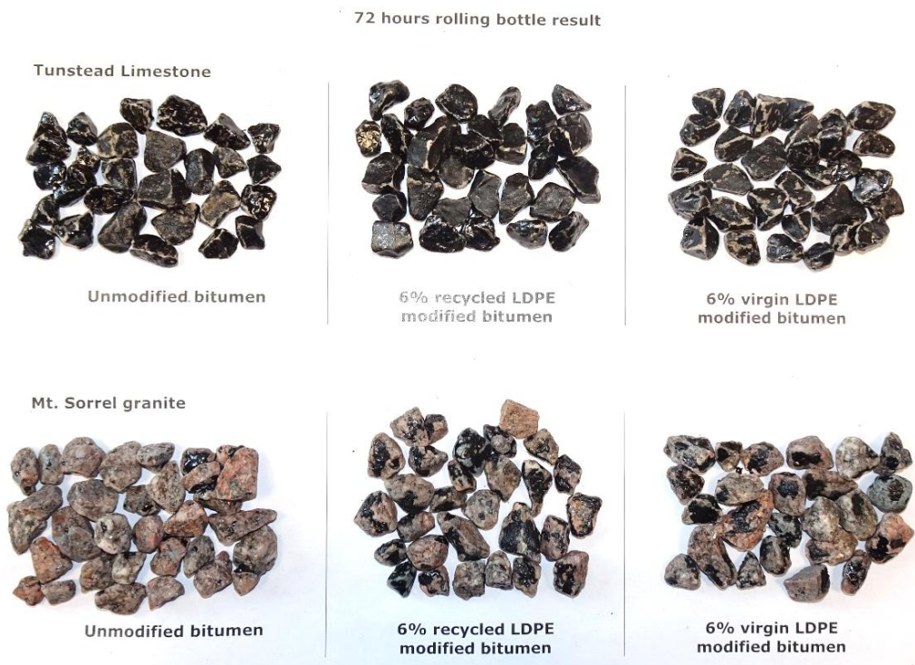
Figure 6. 4: Results of 72 hours rolling bottle test
