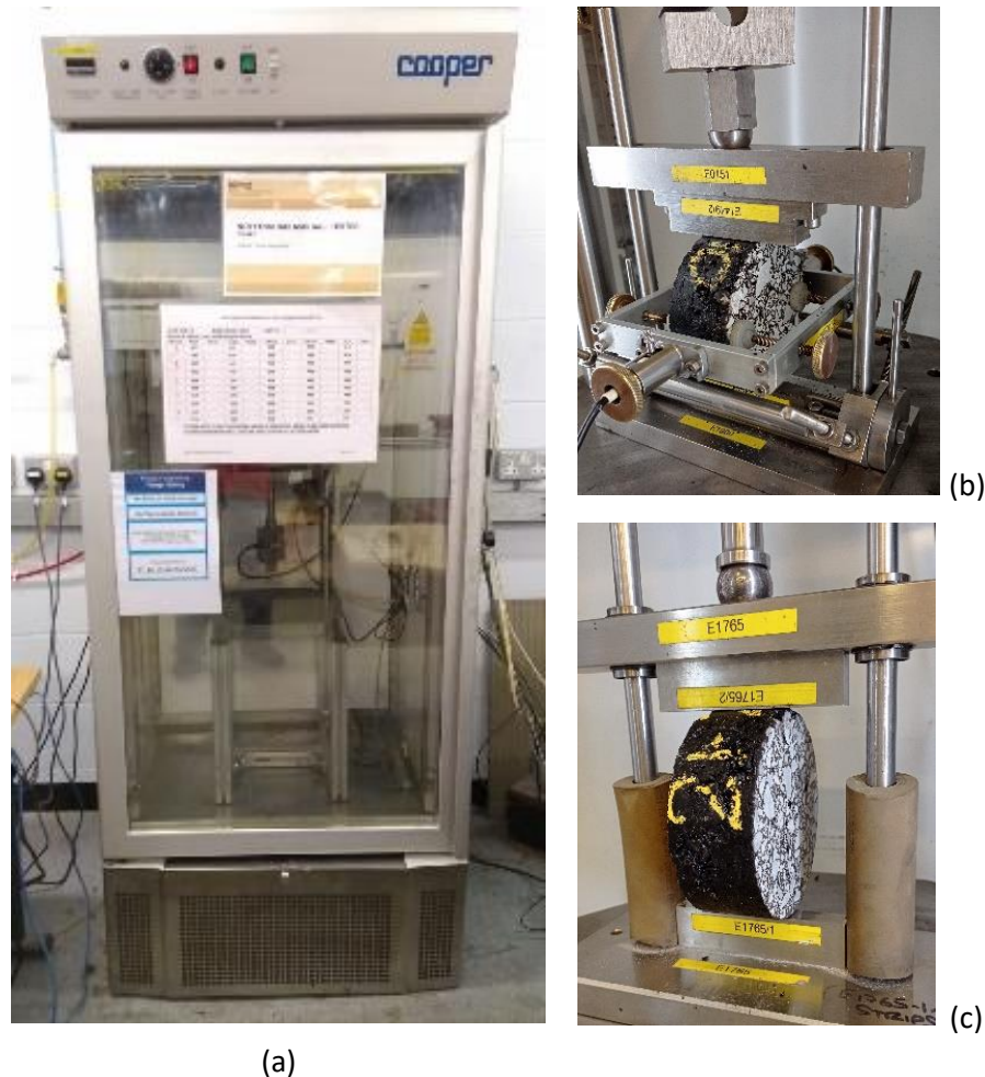
Figure 3. 14: (a) NU-14 (Nottingham Asphalt Tester), indirect configuration for (b) ITST/stiffness and (c) ITFT/fatigue
