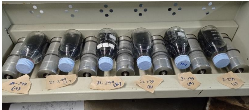
Figure 3. 15: a) Individually spread aggregate mixes for RBT, (b) the RBT settings
