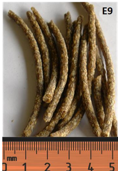
Figure 6-2: Extrudate (E9) from the preliminary extrusion at high moisture content (22%), die temperature (150 °C) and screw speed (400rpm). The appearance of the sample E9 as a cohesive string of material and the small sectional diameter confirmed the poor expansion characteristics.
