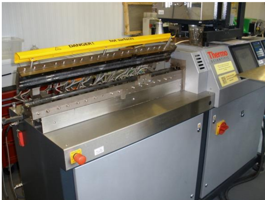
Figure 2-10: Experimental twin screw extruder with barrel section opened.
