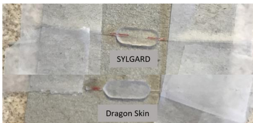
Figure 4.5: Cured sensors from SYLGARD (top) and Dragon Skin (bottom). Sensors are 10mm in length and 4mm in width.
