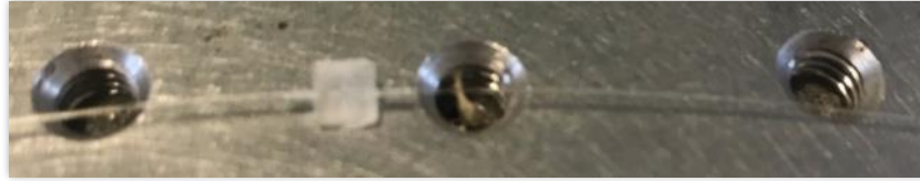
Figure 3.3: A 4mm x 4mm x 1mm cured Vitralit 1655 pressure sensing patch.
