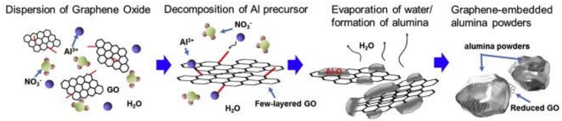
Figure 2.8: Schematic representation for fabricating reduced GO-alumina composite by molecular level mixing process [92].
