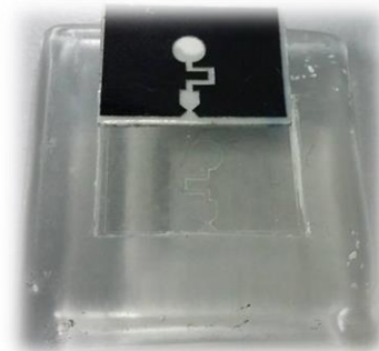
Figure 5.3: Vinyl film master mold with geometry of microthruster design and replicated PDMS soft mold.
