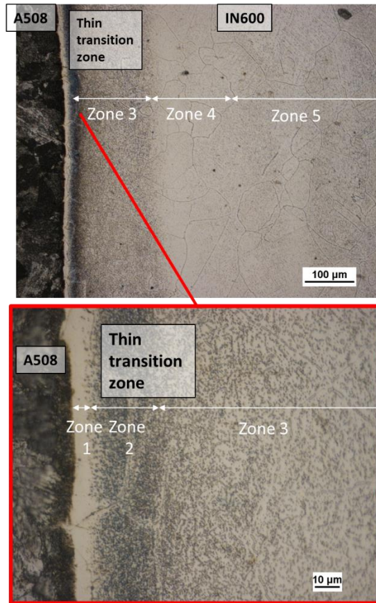
Figure 5.10: Optical micrograph of IN600 alloy side of the interface of A508/IN600 joint in the thin transition zone region.
