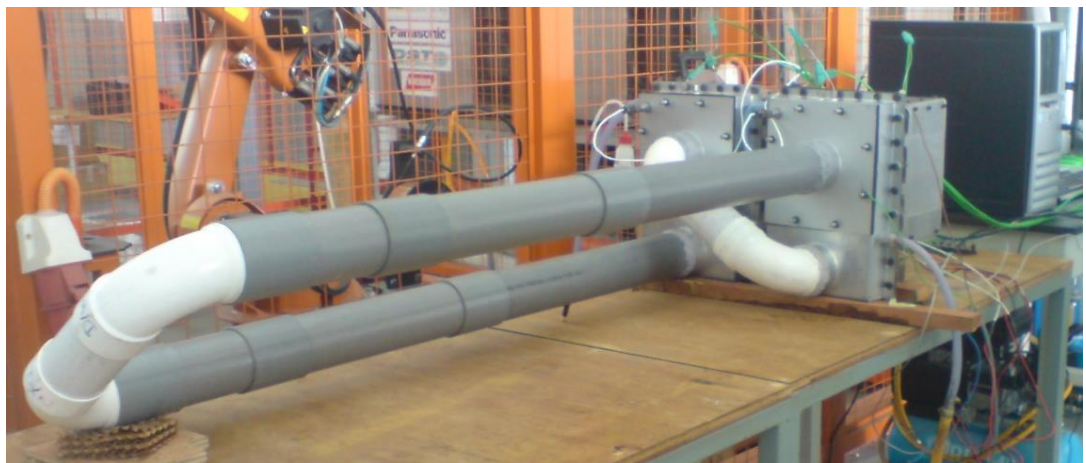
Figure 1.5: The DEMO 2 Engine driven by electrical heaters.
