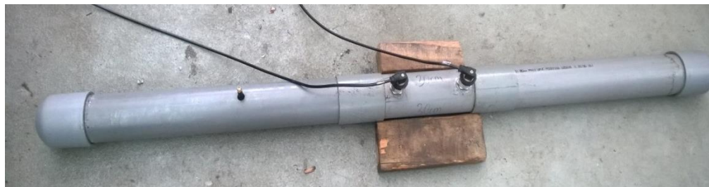
Figure B1: Pressure sensor mountings on the Feedback Loop.
