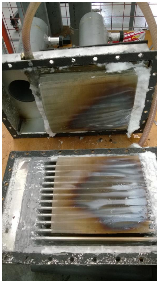
Figure A1: Burnt marks on the regenerator.
