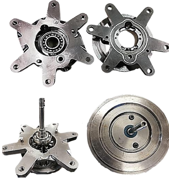
Figure 5.5 Ball bearing retrofit in OTP
