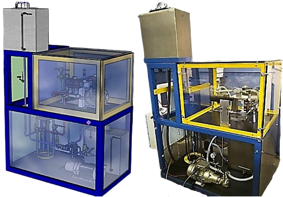
Figure 3.2 Hydraulic rig model design (left) and actual rig (right) of KERB-HAT
