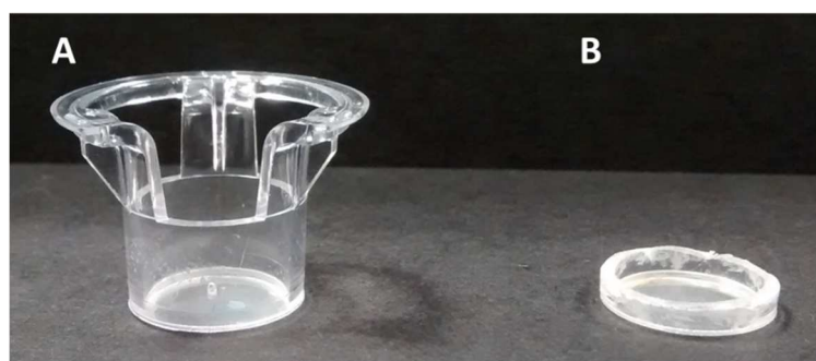
Figure 6.3: modification of the Transwell® insert. A: original Transwell® insert; B: modified Transwell® insert (height = 2 mm)
