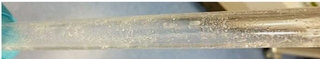
Figure 46: Quartz tube after 0.5 M solution of 17 had been irradiated.
