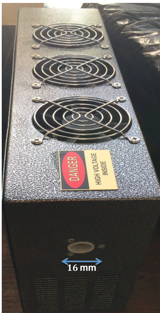
Figure 16: Photograph of the XeBr excimer lamp. All three lamps have the same dimensions, with a central lamp bore of 16 mm.
