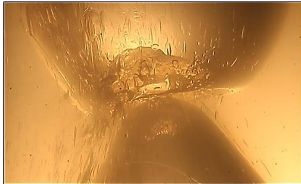
Figure 5.16: A photo of the end and the top of two bubbles at one stage before coalescence in 330 Pa.s Silicone oil and 290 mm diameter column. The gas superficial velocity is 0.009 m/s.
