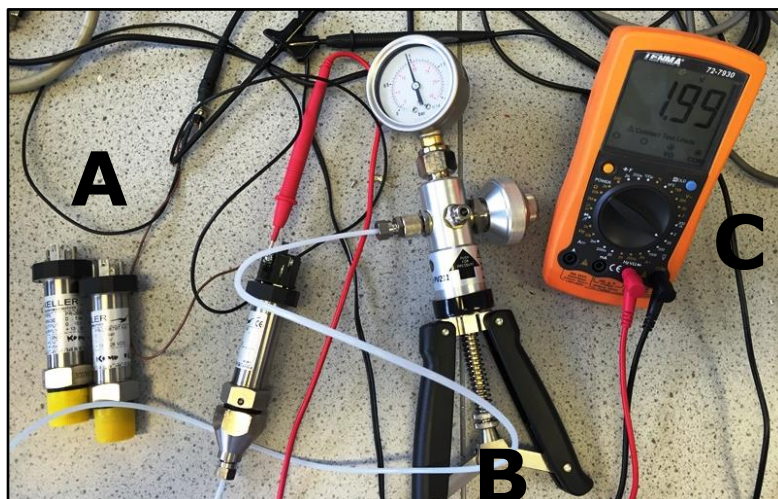
Figure A.6: The pressure sensors bench calibration setup. A is the pressure transmitters, B is the PV211-pneumatic pressure and vacuum pump, and C is the digital Multimeter.
