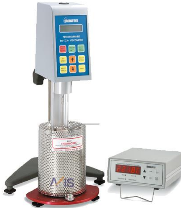
Figure 5.2 The rotational viscometer and ThermoSens used in this investigation
