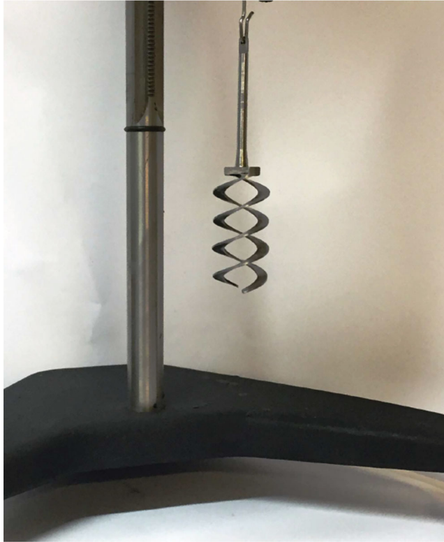
Figure 1. The DHR adapted to a Brookfield rotational viscometer.
