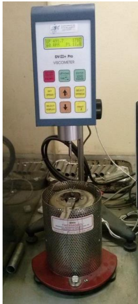
Figure 6.3 The laboratory set-up comprising the Brookfield viscometer and thermosel used to real-time monitoring the CRM binders
