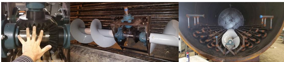
Figure 6.1 An asphalt Rubber Reaction Tanks mounting a helical screw to promote the bitumen-rubber interaction adopted from (D&H Equipment, 2019)
