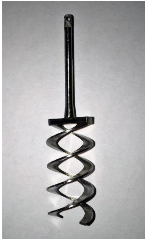
Figure 4.15 The stainless steel DHR impeller for use in a Brookfield Viscometer.
