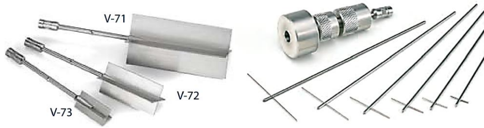
Figure 2.16 Vane Spindles (left) and the T-Bar Spindles with the Helipath stand (right) adopted from (Brookfield, 2015)
