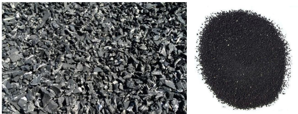
Figure 2.7 Shredded end life tyres (left) and crumb rubber (right)
