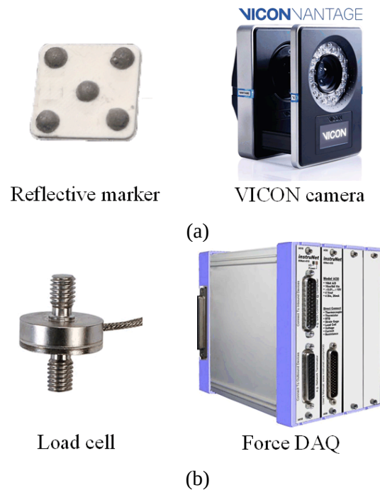
Figure 3-12 The measuring equipment used for the close-loop control of Prototype One and Two: (a) a vision system comprised of multiple VICON cameras for visual feedback; (b) a Load cell and the DAQ (Data acquisition) for sensing the cable tension of the robots.
