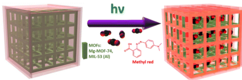
Scheme 1.14 Postsynthetic treatment of MOFs with methyl red to enable photocontrolled carbon dioxide pore access. Reproduced from reference 125.
