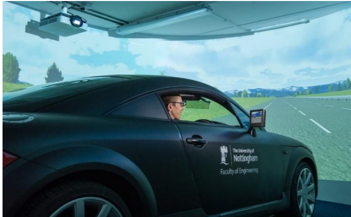
Figure 5-1 University of Nottingham Human Factors Research Group Driving Simulator
