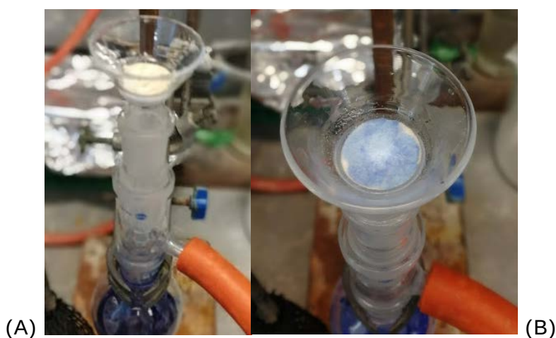
Figure 23: Attempted staining of beads after reacting with ethylenediamine for (A) 5 mins and (B) 2 hours.
