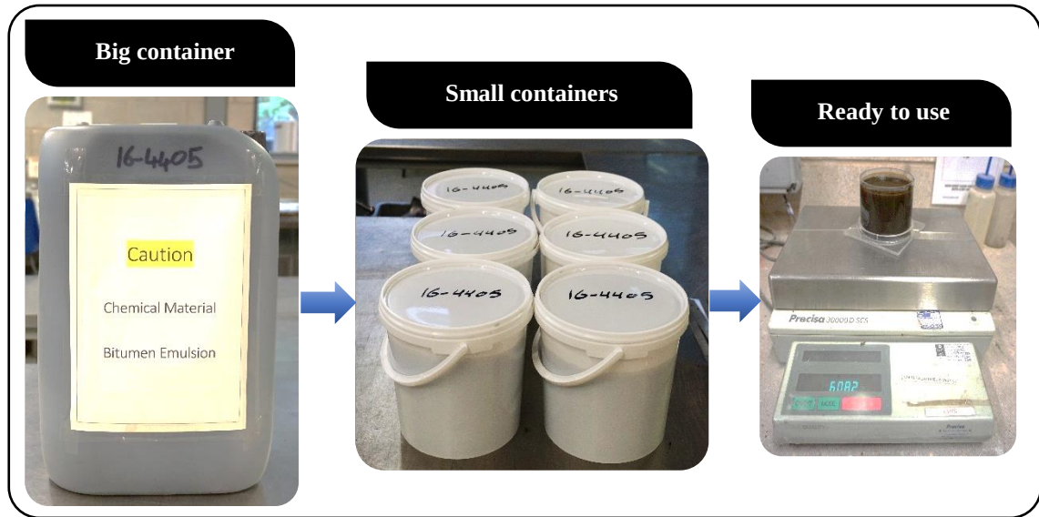
Figure 3.4 Preparing the bitumen emulsion to mix
