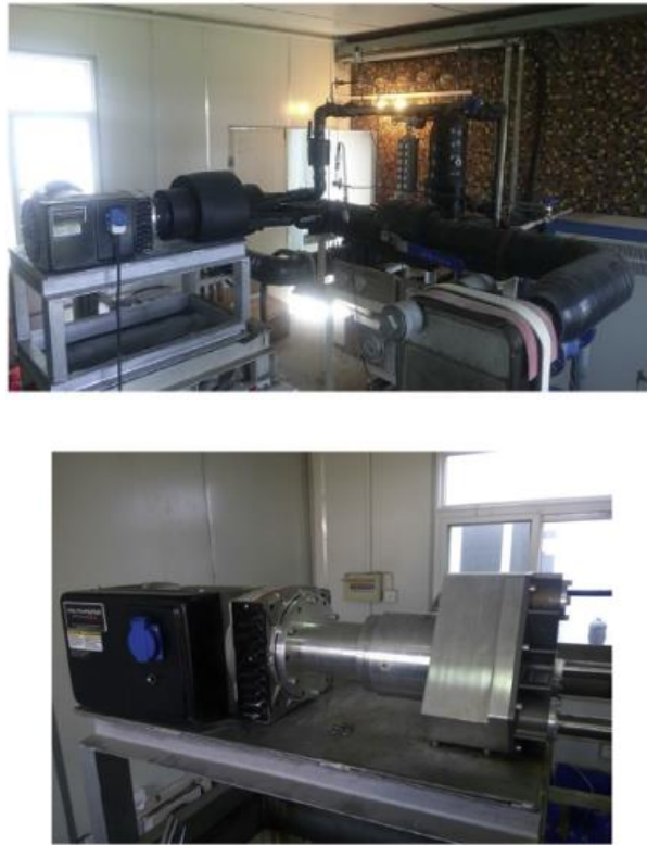
Figure 6.2 Experimental layout and expander-generator coupling
