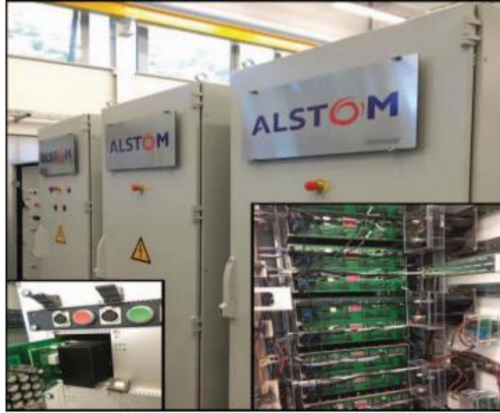
Figure 8.2: The small scale prototype hardware: SM and IGBT module interface PCBs (left), and backplane PCBs (right)[86].
