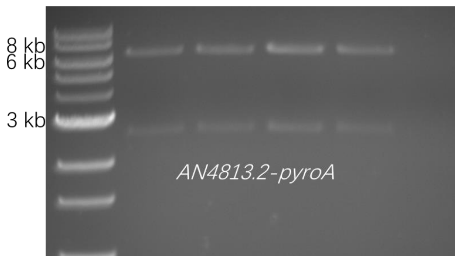
Appendix 35 Selection of the complementation plasmids. The pUC19-AN4813-pyroA plasmids were digested with Sma I, and the complementation cassettes were approx. 7.1 kb.
