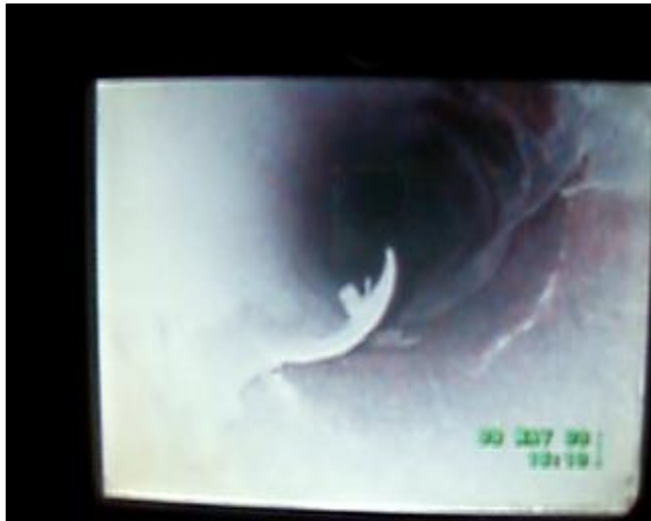
Figure 2.8: Digital photography provided by Doosan Babcock of the spallation on the inside surface of a typical P92 pipe [Chi and Barnard, 2012].
