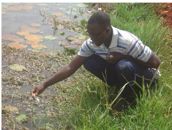
Figure 2.4. Recording of the water temperature of a site using a digital probe thermometer
