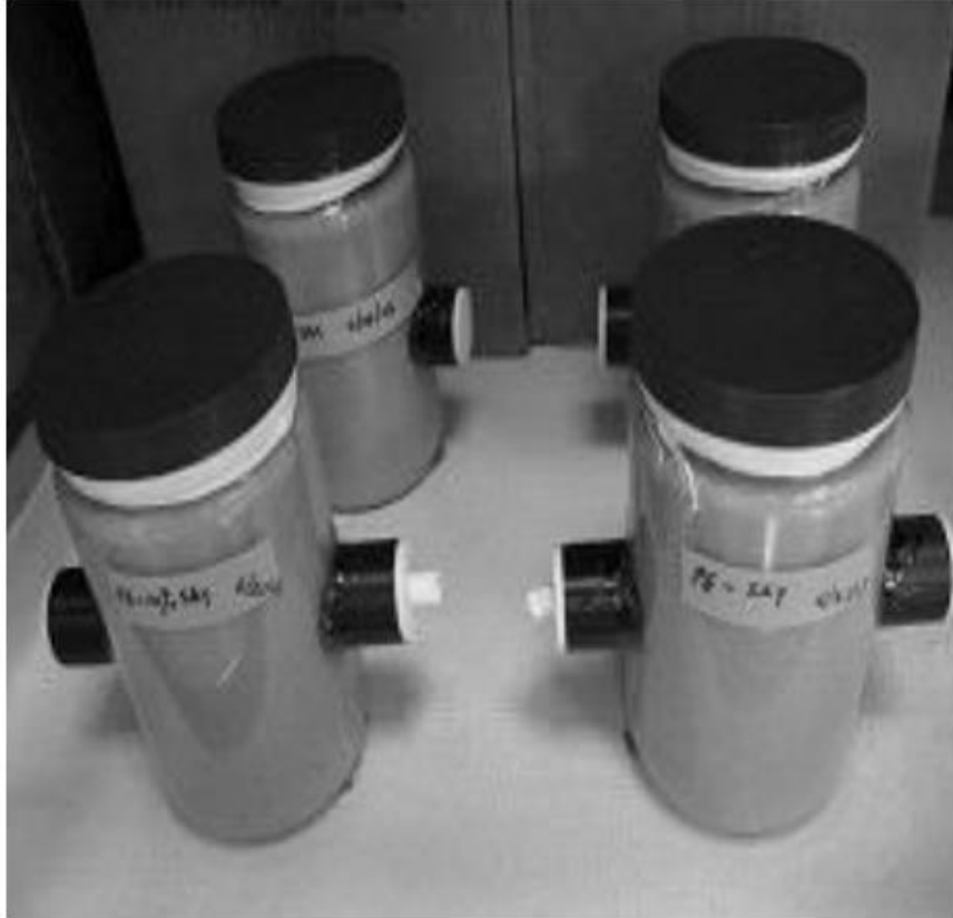
Figure 3 Pipe-bottle apparatus (Ong et al. 2008, Figure 3.1)
